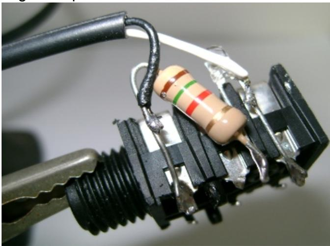
If not using the limiter, just wire white wires to rear jack tabs. And the black wires to the front jack tabs.
