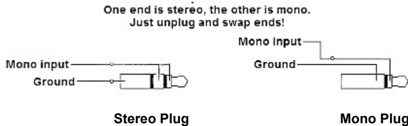
You can now use your headset with either a mono detector or stereo detector by just reversing the plug ends that go into the detector and headset. No need for a stereo/mono switch.
