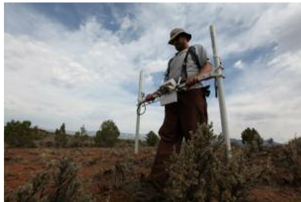
Figure 2. Team Geophysics member Duncan McKinnon collects magnetic gradient data at the Dillard Site, Crow Canyon Archaeological Center, Colorado. Image courtesy of Oregon Public Broadcasting.
